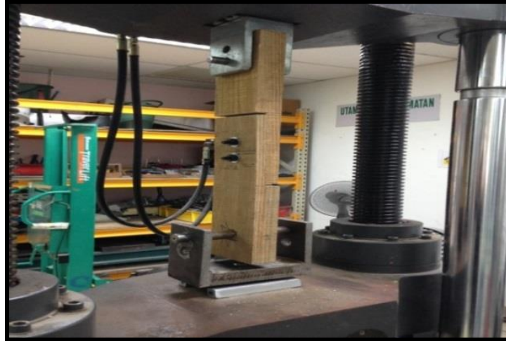
Figure 3 Tensile test set up by using UTM
