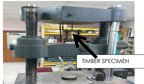
Figure 9 Pull-out strength test set-up (real picture)
