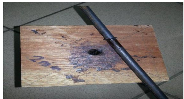
Figure 13 Failure mode of rod interface
