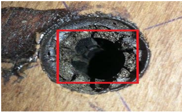
Figure 14 Cracking of adhesive
