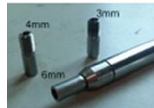
Figure 2 Nozzles of three different sizes (3 mm, 4 mm and 6 mm)
