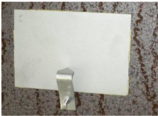
Figure 2 Specimens attached by anchoring device
