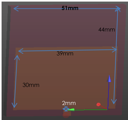
Figure 4 Dimensional view of rectangular microstrip applicator
