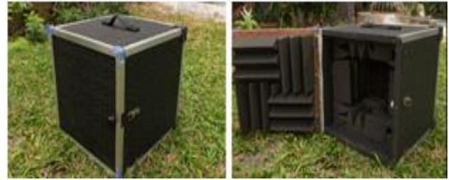
Figure 2 (a) Actual photo of the anechoic chamber (b) Inside of the anechoic chamber
