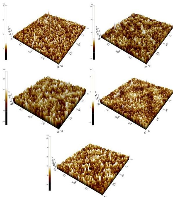
**Figure 4** 3D AFM images of ZnO/TiO<sub>2</sub> bilayer film anneal at (a) 300°C, (b) 400°C, (c) 500°C, (d) 600°C and (e) 700°C
