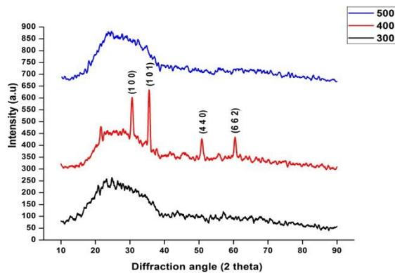
**Figure 5** XRD spectra for ZnO/TiO<sub>2</sub> bilayer film annealed at 300°C, 400° and 500°C respectively
