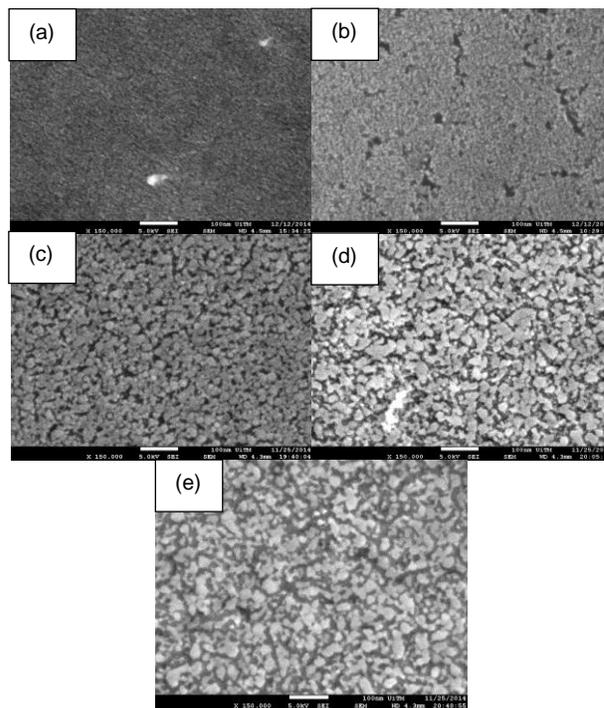
**Figure 2** SEM images for ZnO/TiO<sub>2</sub> bilayer film anneal at (a) 300°C, (b) 400°C, (c) 500°C, (d) 600°C and (e)700°C.
