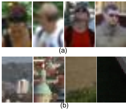
Figure 7 Samples for SVM training with normal orientation: (a) positive samples, (b) negative samples
