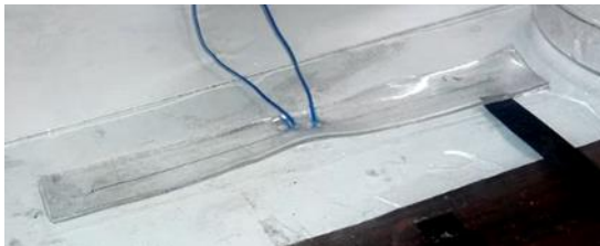
Figure 3 Liquid metal antenna
