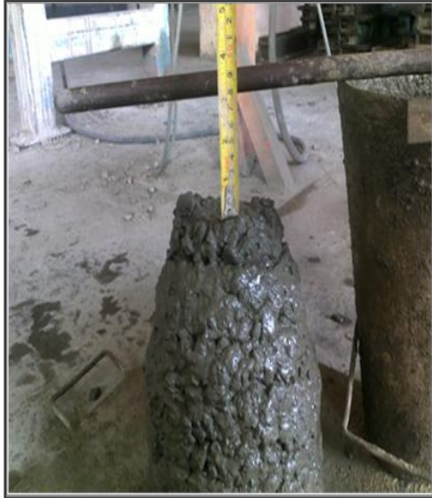
Figure 3b Concrete slump test measurements
