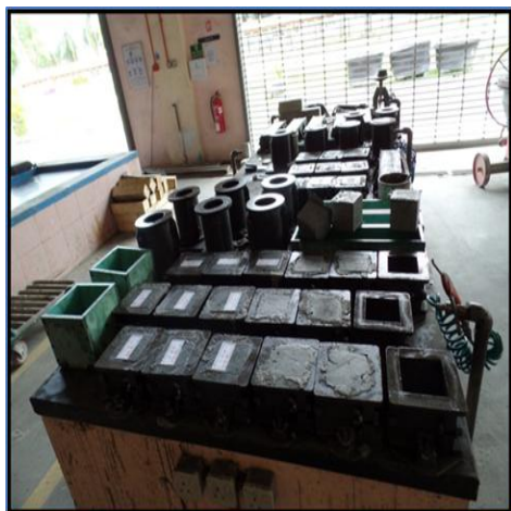
Figure 1 Concrete casting in standard cube moulds
