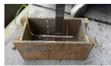
c. Installation of the steel bar
