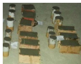
a. Casting of concrete
