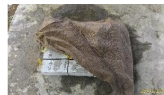
e. Curing of the corrosion specimen
