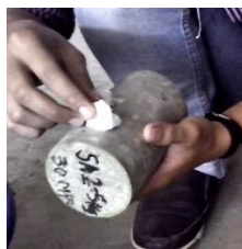
d. Cleaning the specimen until the SSD condition is obtained
