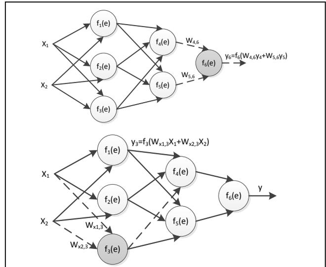
Figure 2 How the signal flow in a neural network [11]
