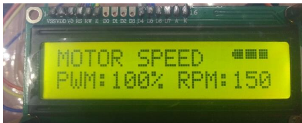
Figure 3 A LCD display of the flicking device indicating the duty cycle of the PWM and speed of the flicking device
