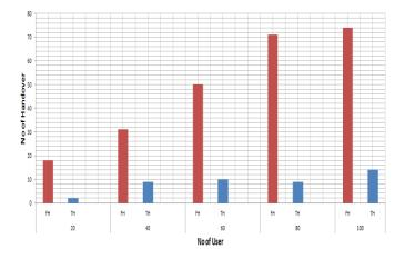
Figure 5 Number of handovers versus number of Users for hand-in handover
