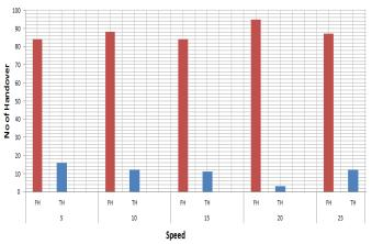
Figure 3 Number of handovers versus Speeds of UE for random movement.
