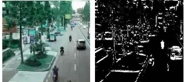
Figure 1 Left side is the current image. The right side is the result image using the EWMA method
