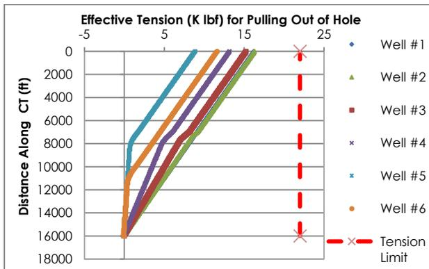
Figure 7 Effective Tension of 1"CT and Tension Limit v.s. distance along CT inside 2.875" Tubing during POOH
