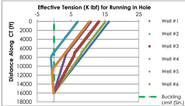
Figure 6 Effective Tension of 1"CT and Buckling Limit v.s. distance along CT inside 2.875" Tubing during RIH
