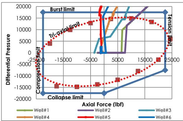
Figure 9 Tension-Pressure plot and the operating envelope for 1" CT in 3.5" tubing of Well #1 - #6
