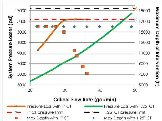
Figure 5 System Pressure Losses and Max depth of intervention v.s. Critical Flow Rate
