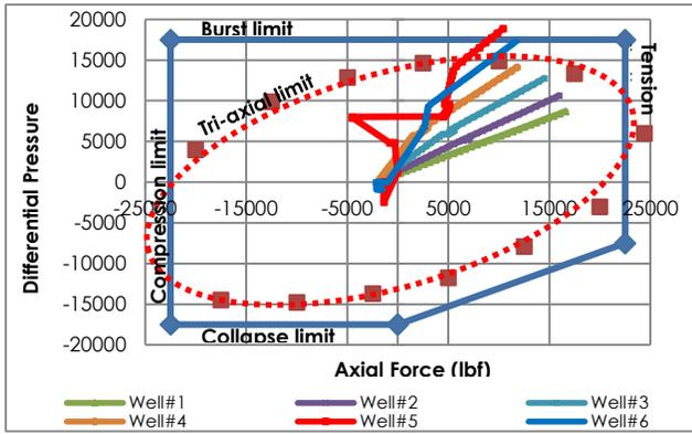
Figure 8 Tension-Pressure plot and the operating envelope for 1" CT in 2.875" tubing of Well #1 - #6
