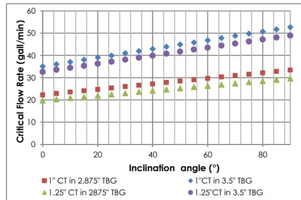
Figure 4 Critical Flow Rate for solid cleanout (milling and sand cleanout applications) in 2.875" and 3.5" tubing
