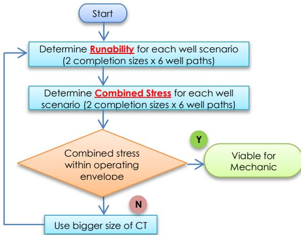
Figure 3 Flowchart for mechanical consideration
