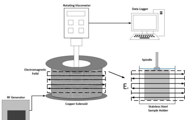
**Figure 2** Schematic diagram of experimental setup for measuring nanofluid viscosity under applied electromagnetic field
