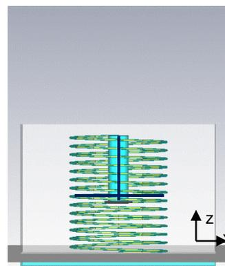
**Figure 1** Heat Simulation model of copper solenoid at 167 MHz
