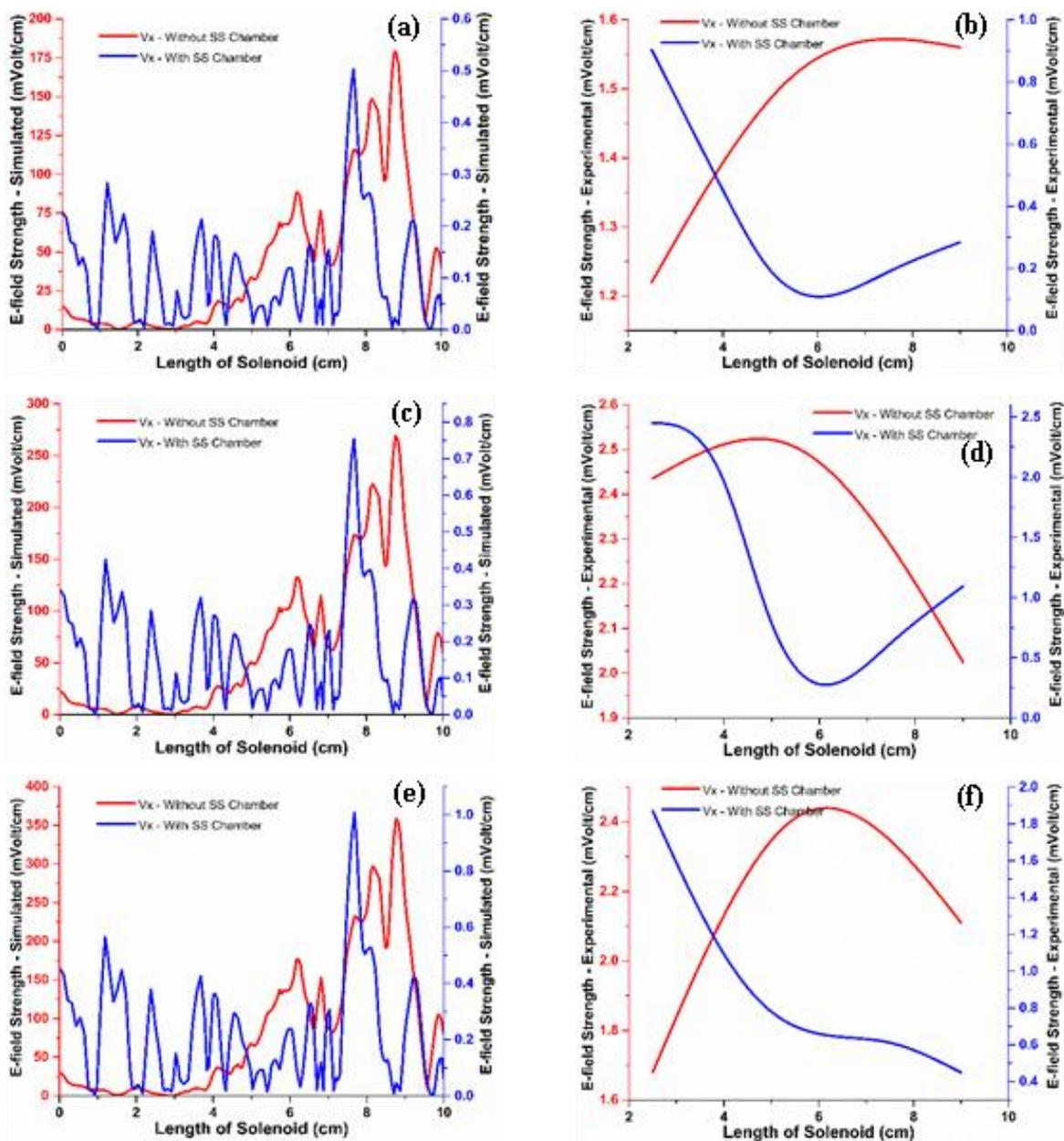
**Figure 3** Comparative results of E-field strength via simulation and experiment at an applied voltage of 1V (a, b), 1.5V (c,d) and 2V (e, f)
