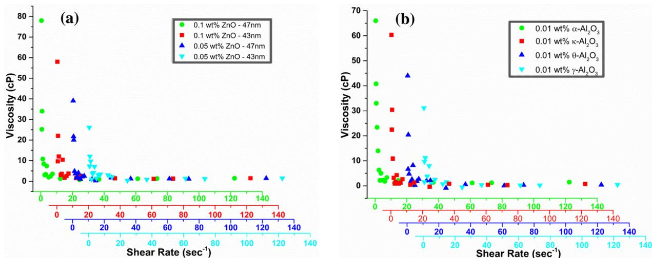
Figure 4 Viscosity versus shear rate of (a) ZnO and (b) Al<sub>2</sub>O<sub>3</sub> nanofluids at different particle concentrations
