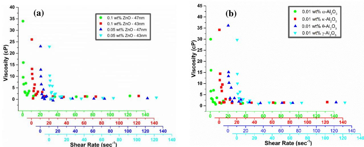
Figure 5 Viscosity versus shear rate of (a) ZnO and (b) Al<sub>2</sub>O<sub>3</sub> nanofluids under applied electromagnetic waves at a applied volatage of 1.5V
