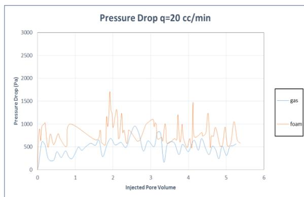
Figure 8 Pressure drop for  $q=20$  cc/min
