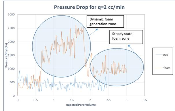
Figure 5 Pressure drop for q=2 cc/min
