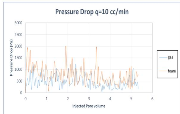
Figure 7 Pressure drop for q=10 cc/min
