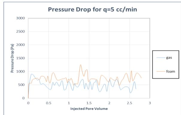
Figure 6 Pressure drop for q=5 cc/min
