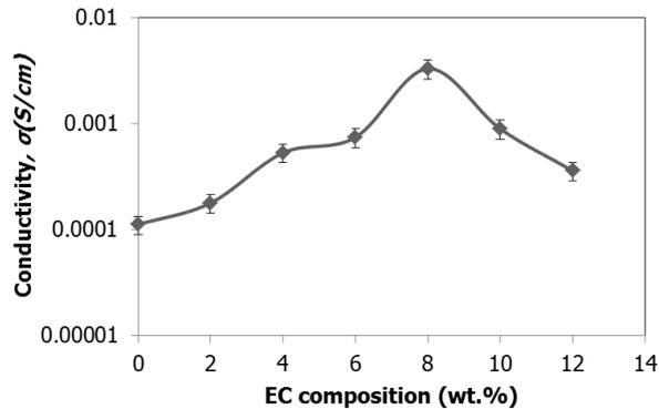
**Figure 1** Ionic conductivity at room temperature as a function of EC composition
