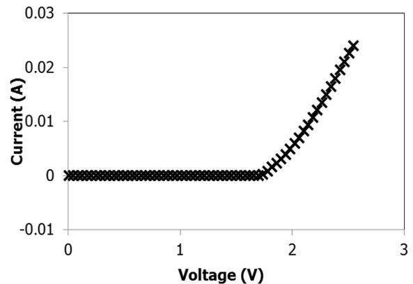
**Figure 3** Linear sweep voltammometry for sample AE8 PSBs system
