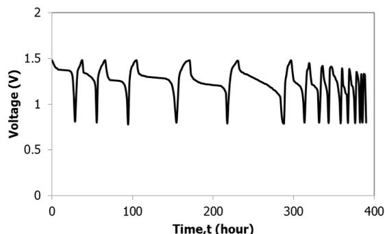
**Figure 6** Discharge-charge curve of PSBs solid-state proton battery
