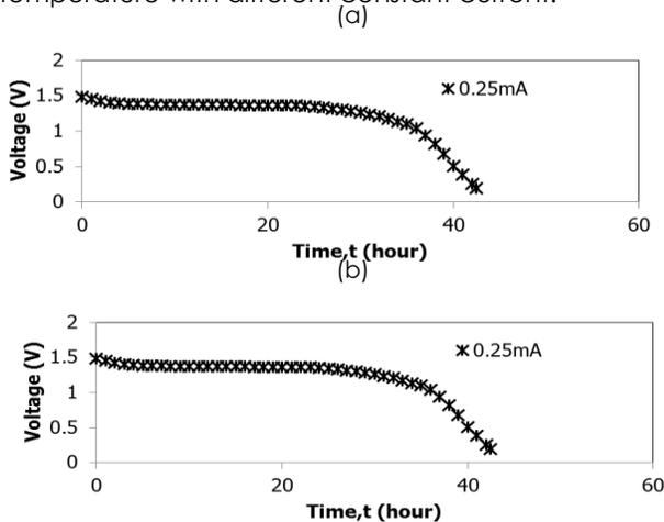
**Figure 5** Discharge characteristics at different constant current for PSBs solid-state proton batteries
