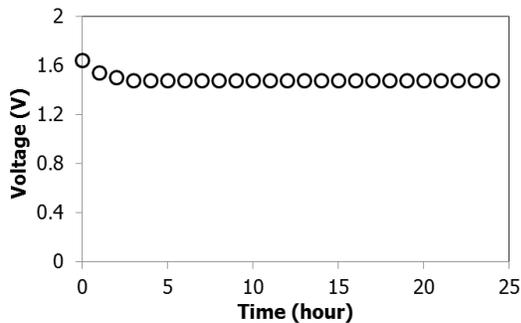
**Figure 4** Open circuit voltage for BPSs solid-state proton battery system
