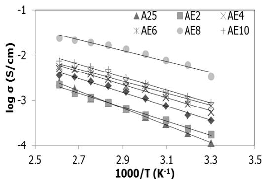
**Figure 2** Temperature dependence of ionic conductivity for PSBs system
