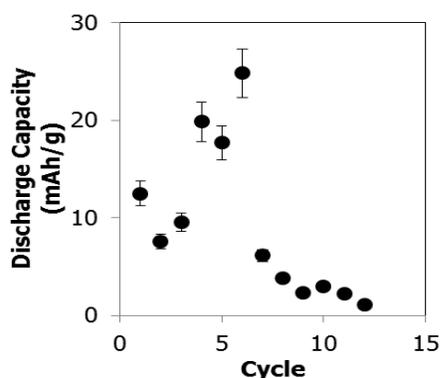
**Figure 7** Discharge capacity for PSBs solid-state proton battery at different cycle
