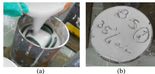
**Figure 1** (a) slurry with optimum viscosity of 9.0 cm (slump test) easily filled the metal flask and (b) slurry hardened forming a block mold
