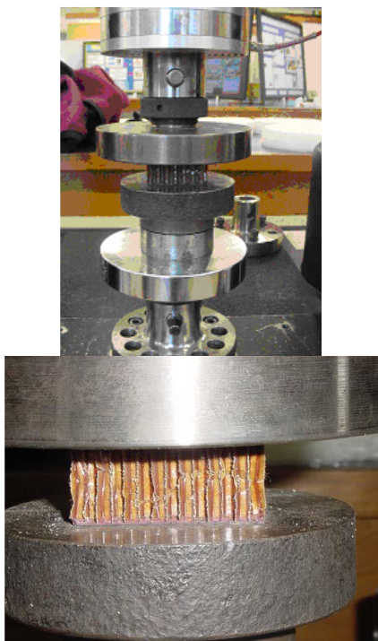
Figure 16 Compression test, showing a fracture line through specimen[18]
