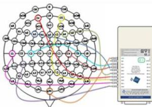
**Figure 2** Locations of the electrode on the 74 channels of g.GAMMAcap2 with eight monopolar channels connected to g.GAMMAbox
