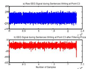
**Figure 5** (a) EEG signal during sentence writing (b) EEG signal during sentence writing after band pass filtering
