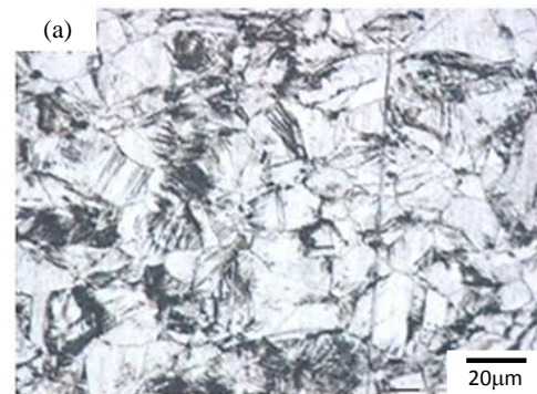
(a) Microstructures of 304 stainless steel sheet of thickness 100 \mu\text{m}
