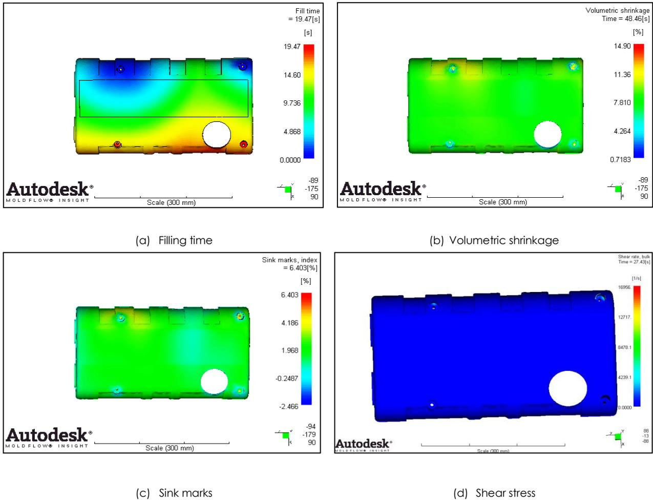
Figure 2 Post-filling stage simulation
