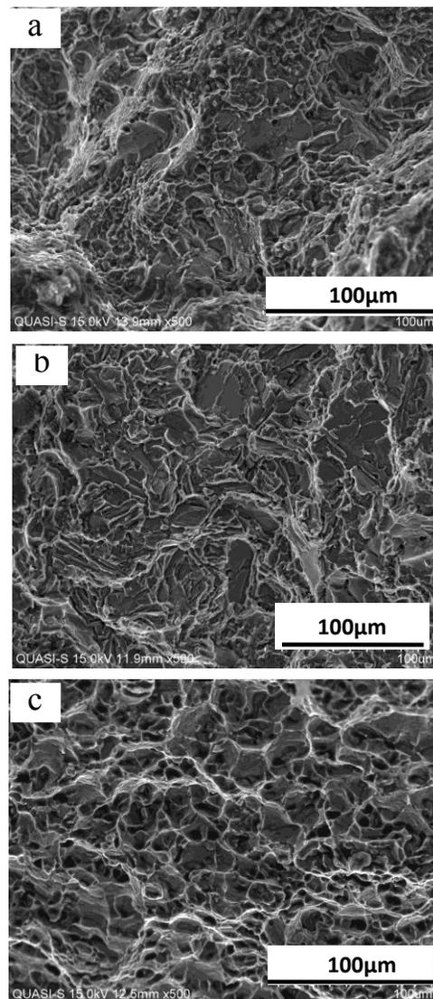
**Figure 6** SEM images of the tensile fracture surface of A356 alloy in different conditions, (a) as received, (b) as rheocast, and (c) as rheocast + T6
