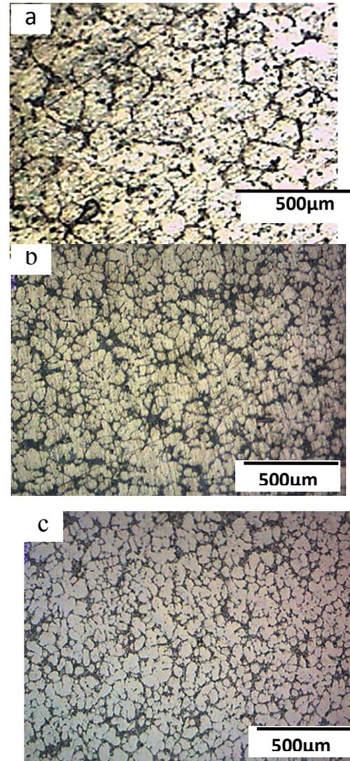
**Figure 5** Microstructures of the thixoformed A356 alloy at different semisolid temperatures, (a) 583 °C, (b) 584 °C and (c) 585 °C
