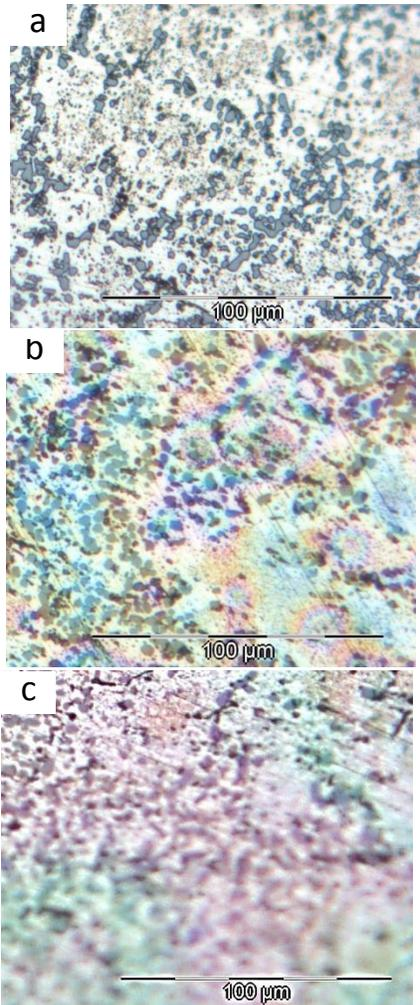
**Figure 4** Microstructures of rheocast samples subjected to T6 heat treatment at different solution heat treatment durations, (a) 2h, (b) 4h and (c) 8h
