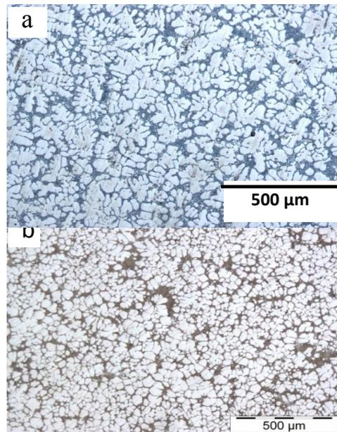
**Figure 3** Microstructure of (a) as received and (b) as rheocast samples
