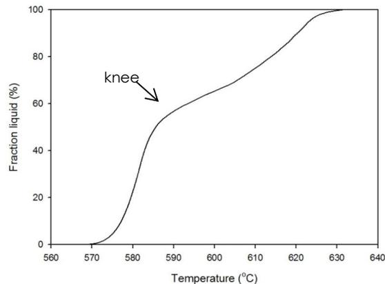
**Figure 1** Curve for liquid fraction versus temperature derived from the DSC
