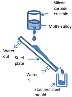
**Figure 2** Schematic illustration of rheocasting [11]
