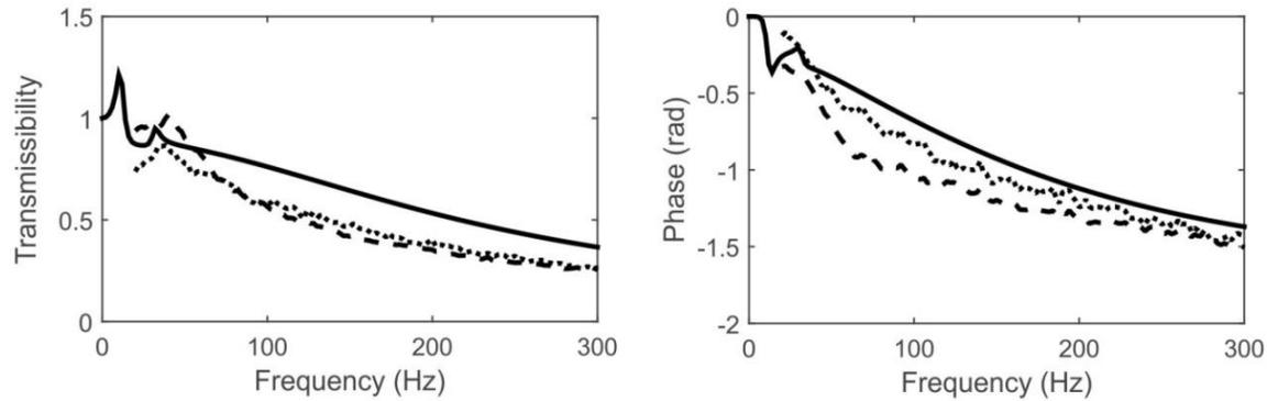
**Figure 3** Transmissibility of the glove material to the palm of the hand (— predicted using model of the hand (this study), ..... predicted using mechanical impedance model, - - - measured) [5].
