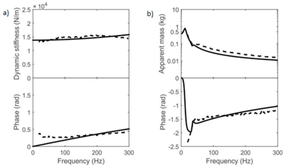
**Figure 2** a) fitted and measured dynamic stiffness of the glove material, b) fitted and measured apparent mass at the palm of the hand (— fitted, - - - measured).
