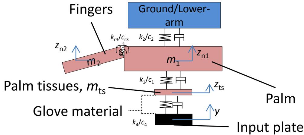
Figure 1 A three degree-of-freedom model the glove and the hand
