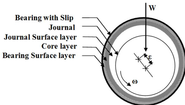
**Figure 1** Geometry of three-layered journal bearing with slip
