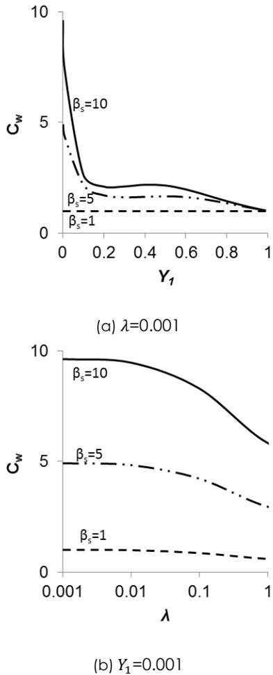
**Figure 3** Load capacity coefficient ( $C_w$ ) of two-layered journal bearing with slip
