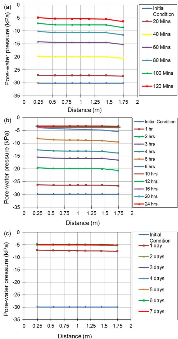
**Figure 9** Suction variation with distance along the interface without transport layer (a) 2-hr (b) 24-hr & (c) 7-day rainfall patterns
