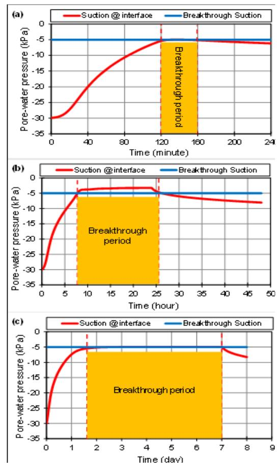
Figure 7 Suction variation at interface without transport layer (a) 2-hr (b) 24-hr & (c) 7-day rainfall patterns
