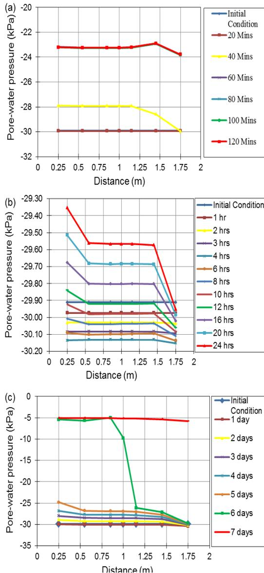
**Figure 10** Suction variation with distance along the interface with transport layer (a) 2-hr (b) 24-hr & (c) 7-day rainfall patterns
