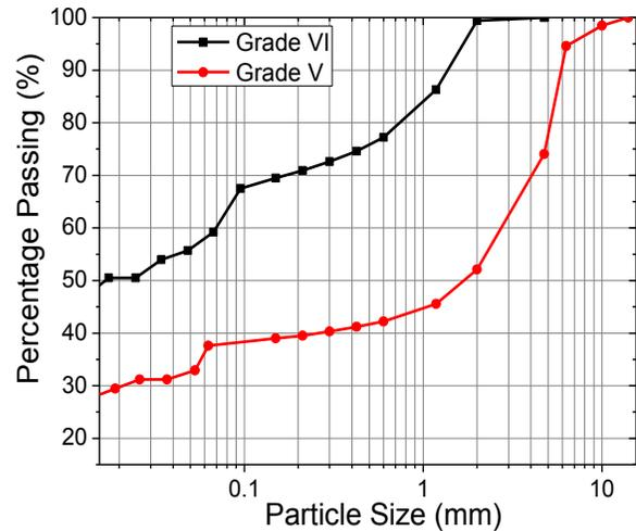
Figure 1 Particle Size Distribution Curves of the soil
