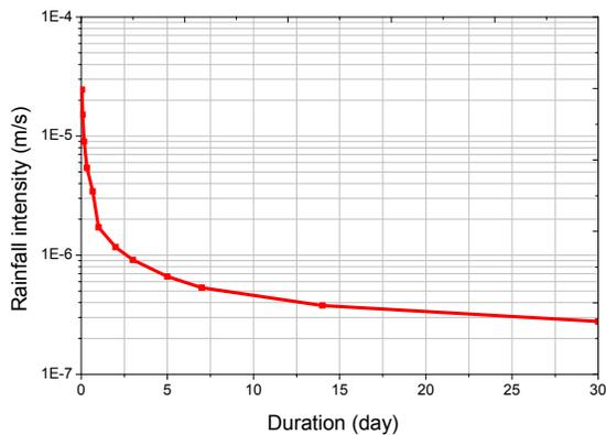
Figure 6 Intensity-Duration-Frequency (IDF) curve of Johor Bahru, Malaysia drainage cell
