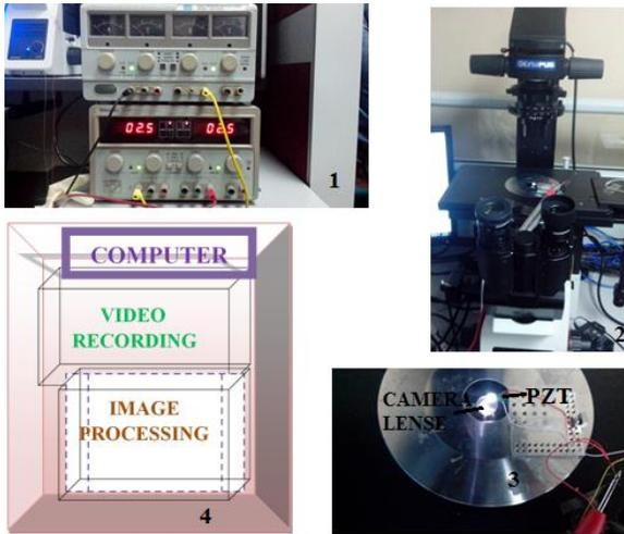
**Figure 1** Section 1 is DC voltage generator. Section 2 is inverted microscope. Section 3 presents PZT actuator focused by camera. Section 4 is image and video processing using computer. The actuator is supplied with DC voltage directly from DC power supply and the corresponding images are captured at different voltage. The images and videos are stored in a computer system.
