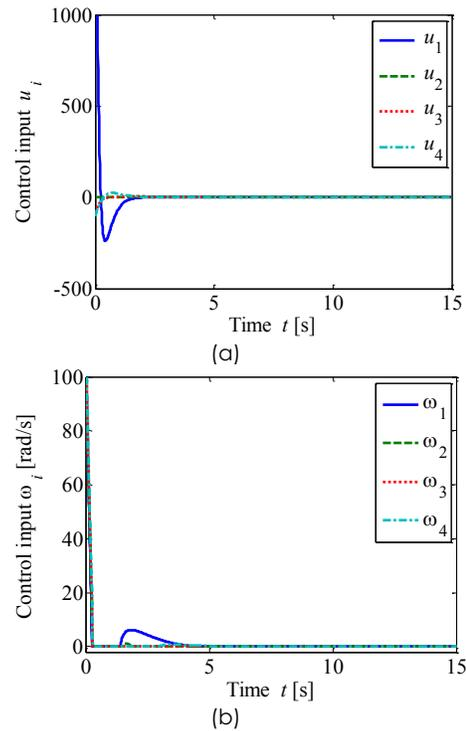
**Figure 7** Optimal parameter values using PSO: (a) A control inputs (b) A control inputs in rotation
