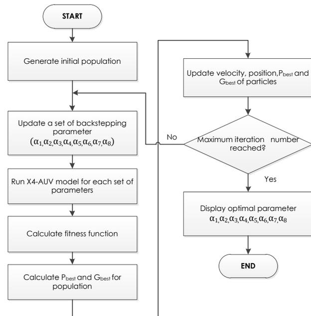
Figure 3 The flowchart of PSO for determining backstepping controller parameters
