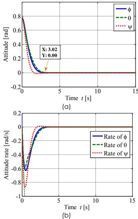
**Figure 5** Optimal parameter values using PSO: (a) Attitude control (b) Attitude rate control
