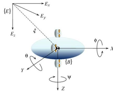
Figure 1 Coordinate systems of AUV
