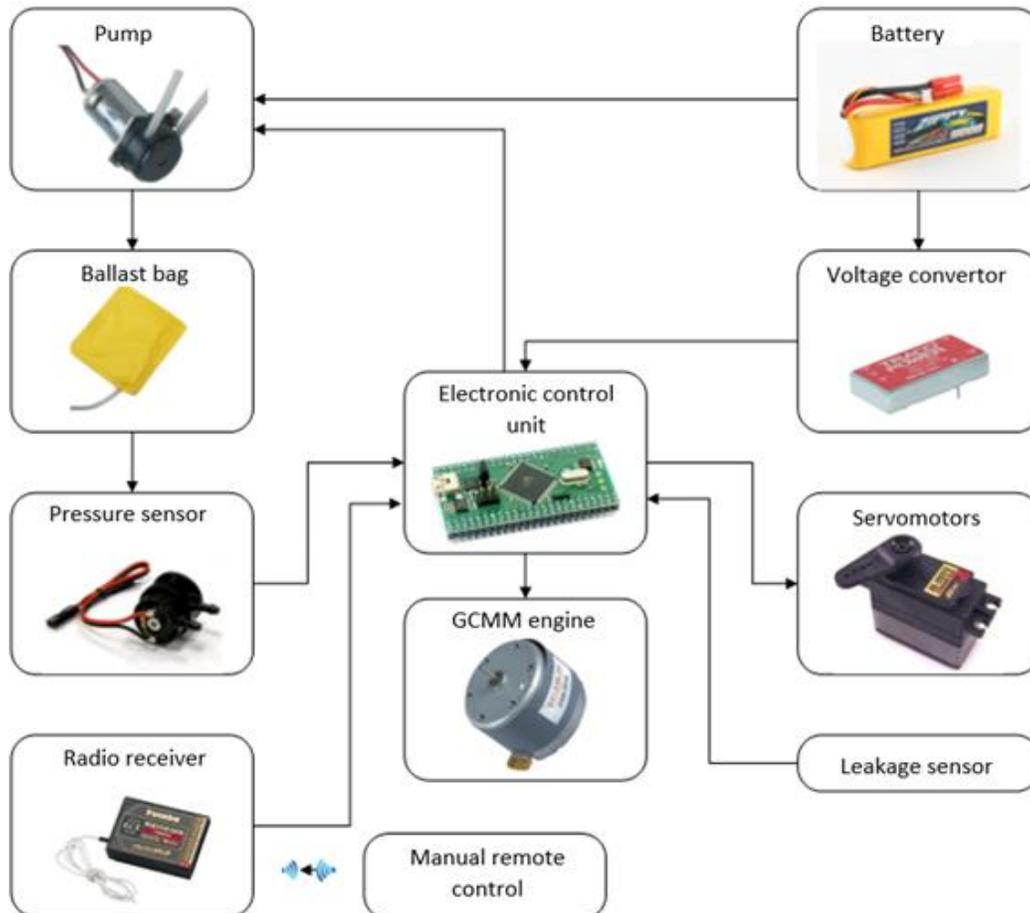
Figure 4 Block diagram of the glider
