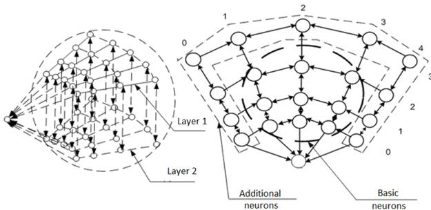
Figure 2 Structure of a multi-layered control neural network
