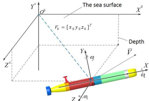
Figure 3 Coordinate systems  $K(OX^0Y^0Z^0)$  and  $K(OX Y Z)$
