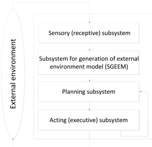
Figure 1 Structure of intellectual control system of AUV
