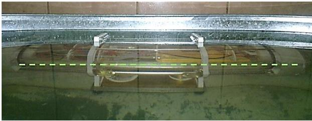
Figure 7 Glider with weight in neutral position
