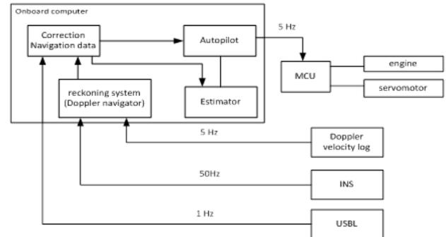
Figure 5 Block diagram of control system prototype
