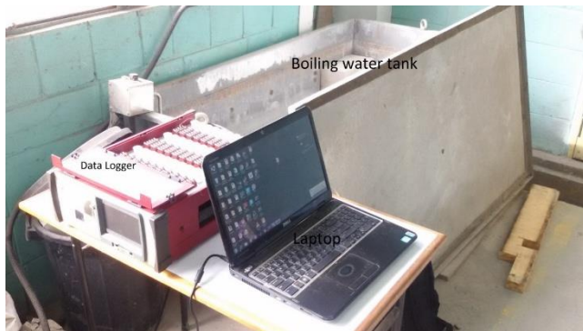
Figure 2 Equipment of heat transfer test
