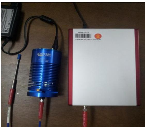
(a) The NIR spectroscopy setup
