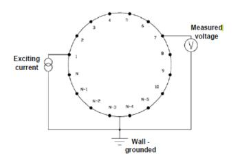
Figure 5 The conducting boundary measurement strategy [11]
