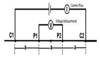
Figure 6 Layout of Wenner-alpha configuration [20]
