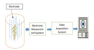
Figure 1 The process of tomography for root detection
