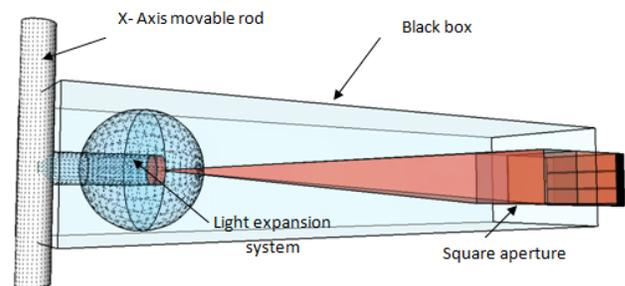
**Figure 2** Laser diode expansion system box
