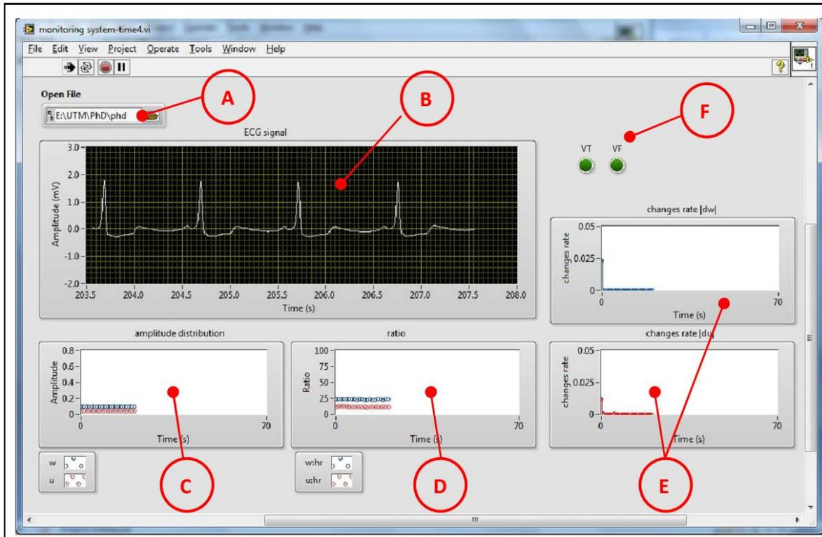
Figure 1 The VI's front panel of CODS
