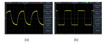
Figure 3 Examples:(a) the exponentially increase pulse shape, (b) approximately 50% duty cycle square wave
