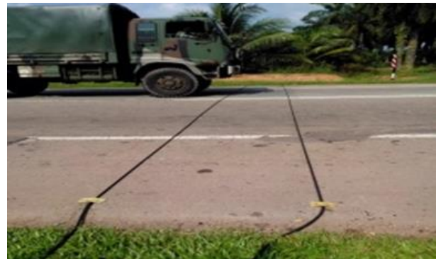
Figure 2 Pneumatic Tubes are 1 Metre Apart
