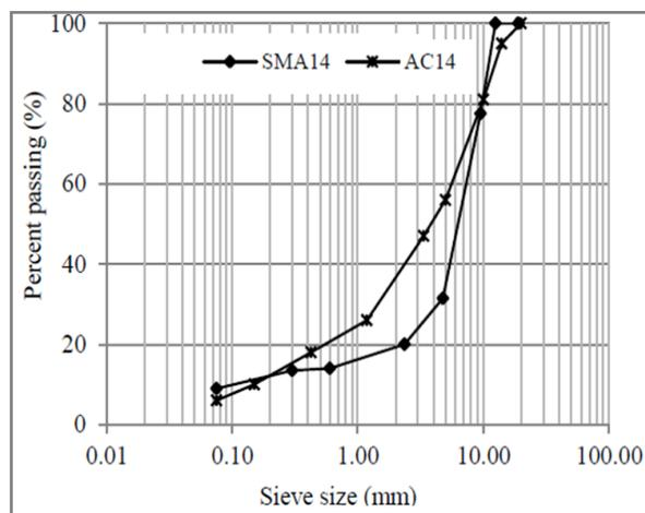
**Figure 1** Aggregate Grading of AC14 and SMA14
