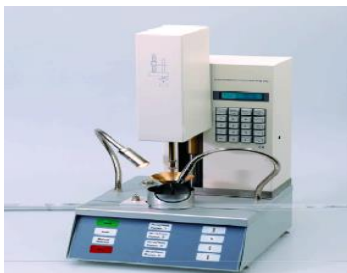
Figure 2 Penetration test setup
