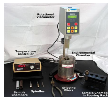
Figure 4 Rotational Viscometer used to determine the viscosity of bitumen
