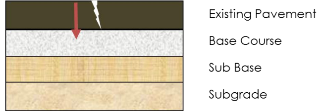
Figure 4 Top-down Crack Propagation in Pavement
