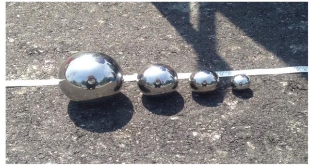
Figure 1 Steel balls with different diameters and masses, m , used in this test
