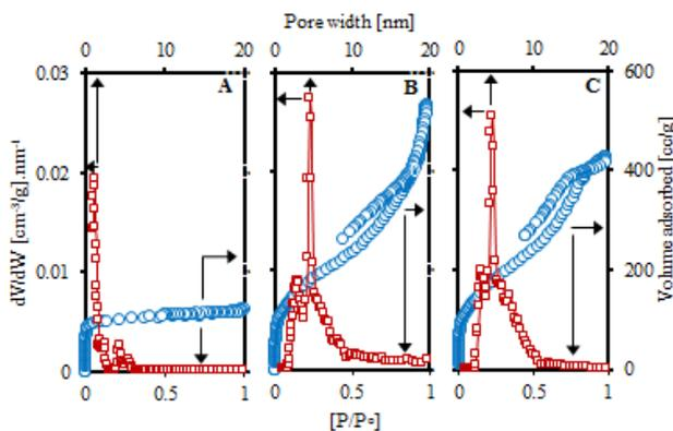
**Figure 1** Nitrogen adsorption isotherms of and average pore width of (A) MoO<sub>3</sub>-HZSM-5 (B) MoO<sub>3</sub>-MSN (C) MoO<sub>3</sub>-MCM-41 obtained from NL-DFT method.
