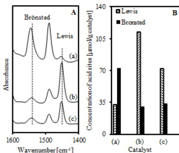
**Figure 2:** FTIR spectra of pyridine adsorbed on (a) MoO<sub>3</sub>-HZSM-5, (b) MoO<sub>3</sub>-MSN and (c) MoO<sub>3</sub>-MCM-41, activated at 673 K, followed by pyridine adsorption at 423 K and outgassed at 423 K. (B) Gaussian deconvolution area of Brønsted and Lewis acid site of (a) MoO<sub>3</sub>-HZSM-5, (b) MoO<sub>3</sub>-MSN and (c) MoO<sub>3</sub>-MCM-41.
