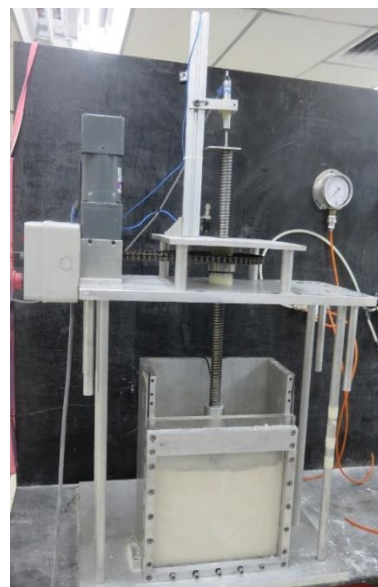
Figure 4 Set-up for the load tests
