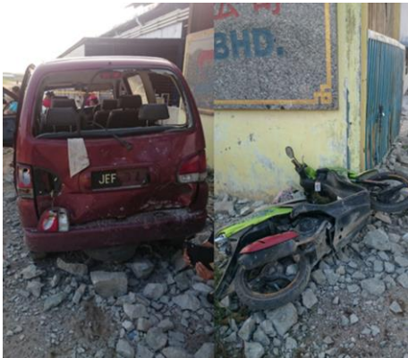
Figure 3 The effect of damage – Vehicles damaged (150 m from the blasting site)
