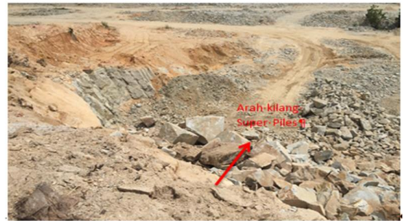
Figure 11 Share of first hole that destroyed – believed to cause fly rock
