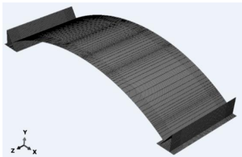
Figure 3 Mesh generation for segment and support designation
