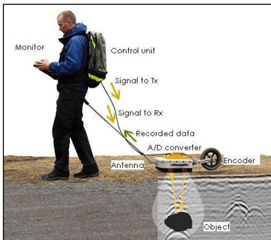
**Figure 10** Principle of GPR survey [13]
