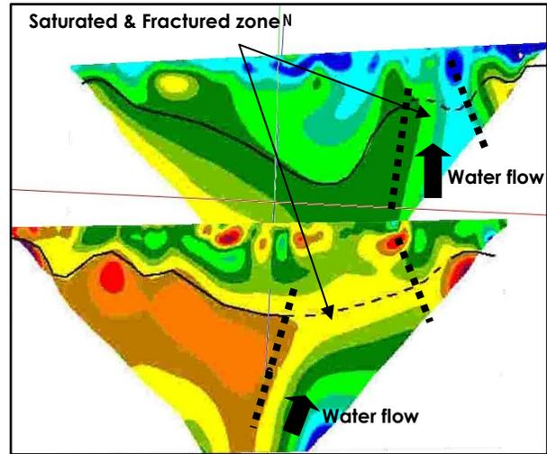
Figure 4 2-D resistivity sections in 3D view and groundwater flow
