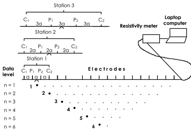
Figure 1 The arrangement of electrodes for 2-DRI survey and the sequence of measurement used to build up a pseudosection [7]
