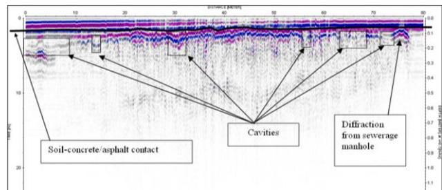
**Figure 11** Radargram section showing GPR data along L1
