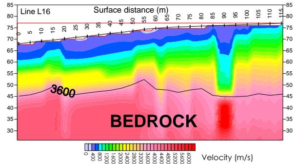
**Figure 8** Interpreted seismic cross section of line L16
