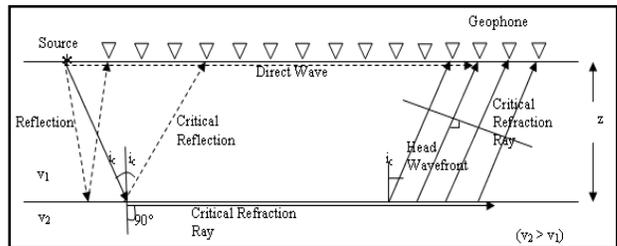
Figure 5 Direct wave, reflection and refraction ray [11]
