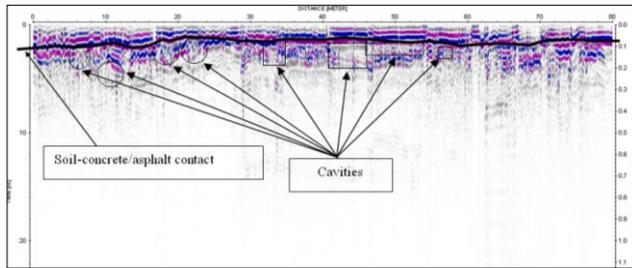
Figure 12 Radargram section showing GPR data along L2
