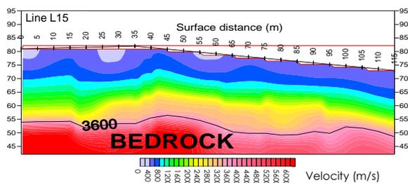
**Figure 7** Interpreted seismic cross section of line L15
