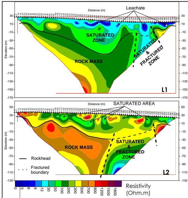
Figure 3 2-D resistivity cross section of line L1-L2 with interpretation
