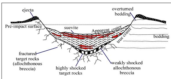
Figure 1 A schematic cross-section of simple crater [2]
