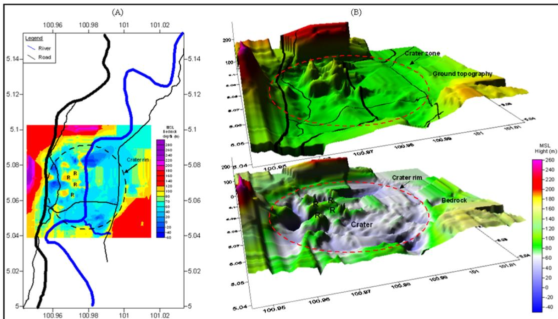
Figure 11 Resistivity topography map of bedrock with crater rim and rebound effect (R): a) 2-D view of bedrock depth, b) 3-D view of bedrock depth
