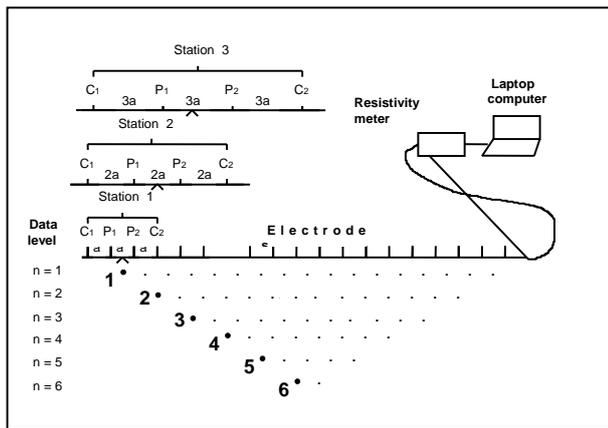
Figure 4 The arrangement of electrodes for a 2-D electrical survey and the sequence of measurement used to build up a pseudosection [8]
