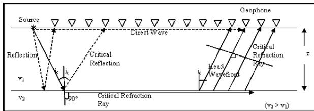
Figure 5 Direct wave, reflection and refraction ray in seismic refraction study [9]
