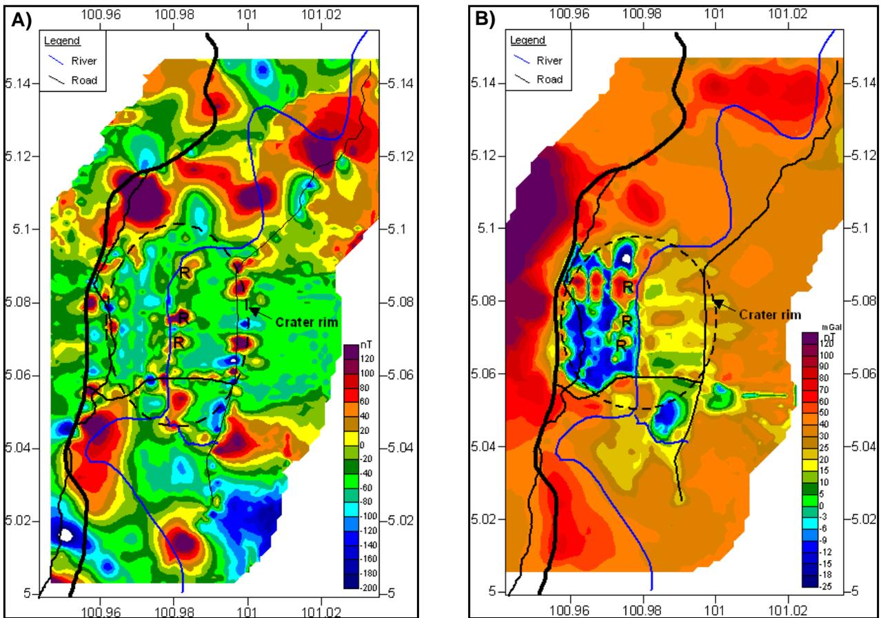
Figure 10 Contour map: a) magnetic residual, b) bouguer anomaly of Lenggong, Perak
