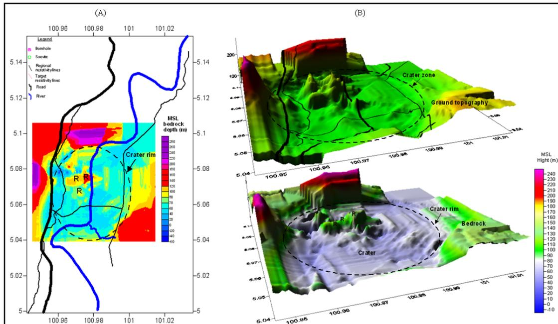
**Figure 12** Seismic topography map of bedrock with crater rim and rebound effect (R); a) 2-D view of bedrock depth, b) 3-D view of bedrock depth
