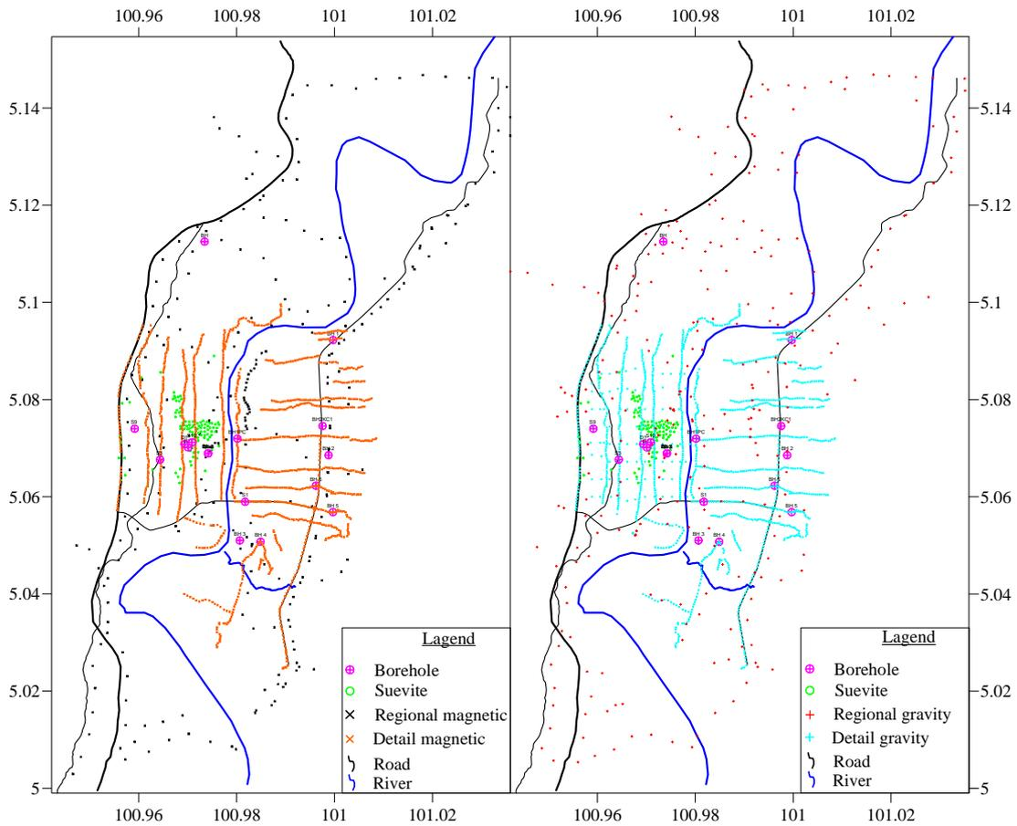
Figure 8 Magnetic and gravity stations at Bukit Bunuh, Perak for regional and detail study.
