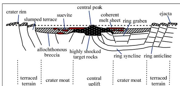
Figure 2 Schematic cross-section of complex crater [2]
