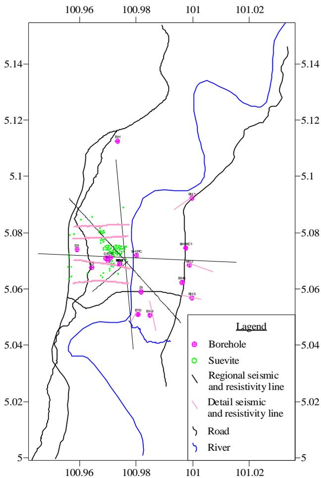
**Figure 9** Seismic refraction and 2-D resistivity survey lines at Bukit Bunuh, Perak for regional and detail study
