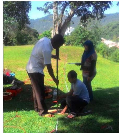
Figure 3 The resistivity and mackintosh probe data ecquisition
