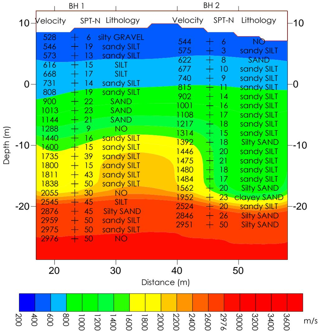
Figure 4 Subsurface velocity distribution of SRT,  $V_p$  and SPT-N value for BH1 and BH2 together with soil lithology at interval of 1.5 m
