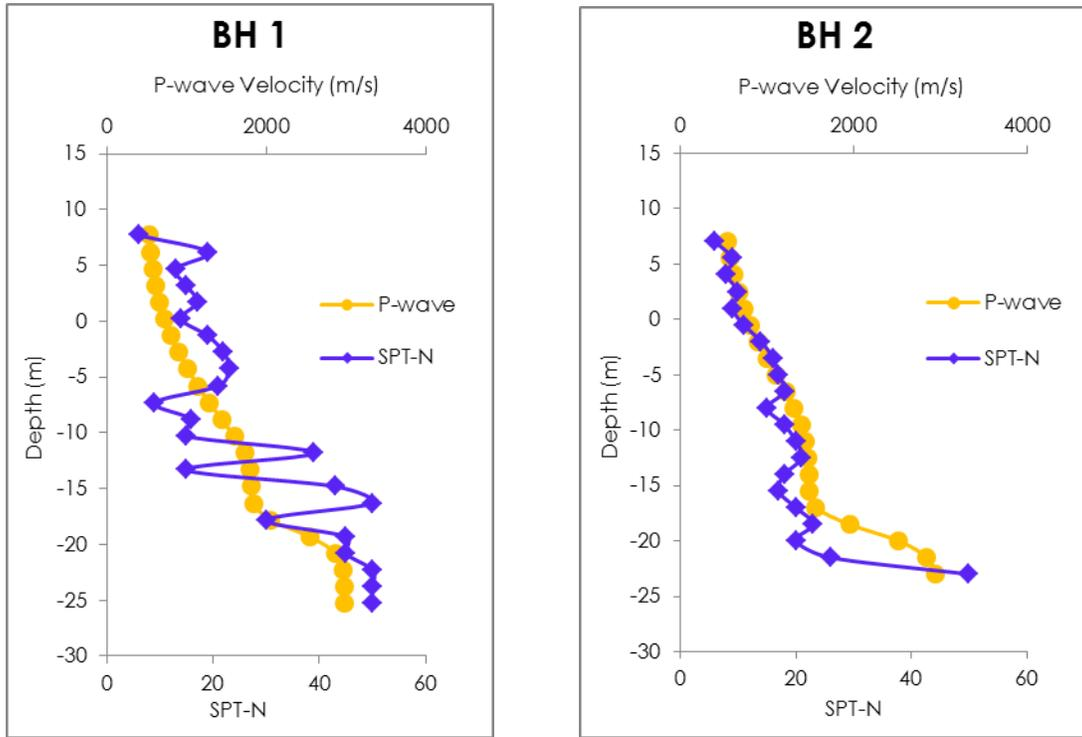
Figure 5 Relationship between  $V_p$  and SPT-N values with depth for BH 1 and BH 2
