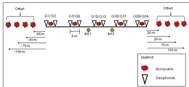
Figure 2 Schematic diagrams of shot points for seismic survey
